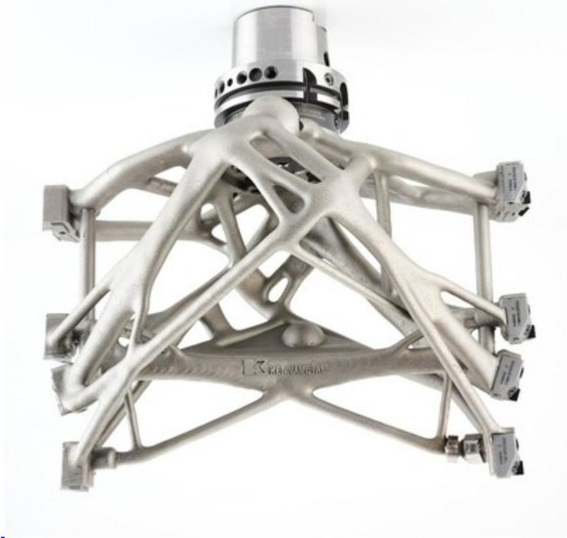
The innovative tool mimics organic shape adaptations observed in nature. The result is a tool that is 45% lighter and has demonstrated a reduced machining time by approximately 50% compared to a conventional solution for the targeted customer. The technology is poised to enhance productivity and efficiency for customers, particularly in the precision machining of components for transportation applications.
