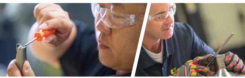
An engineer is securing the drilling insert to a prototype of WIDIA's new Top Cut Four indexable drilling platform.
